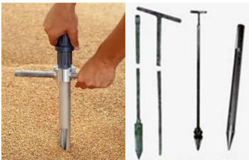
1-rasm. Don shuplari va cho'mich. 1-vagon konus shuplari; 2-qop shupi; 3- silindr shup; 4-cho'mich
